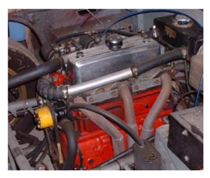
Foam single filters were fitted as the unitary style were too big to clear the passenger side footbox, and I didn't wish to start hacking that about and losing originality. As the front inner fenders were left off the car to improve accessibility, filtering is especially important!
